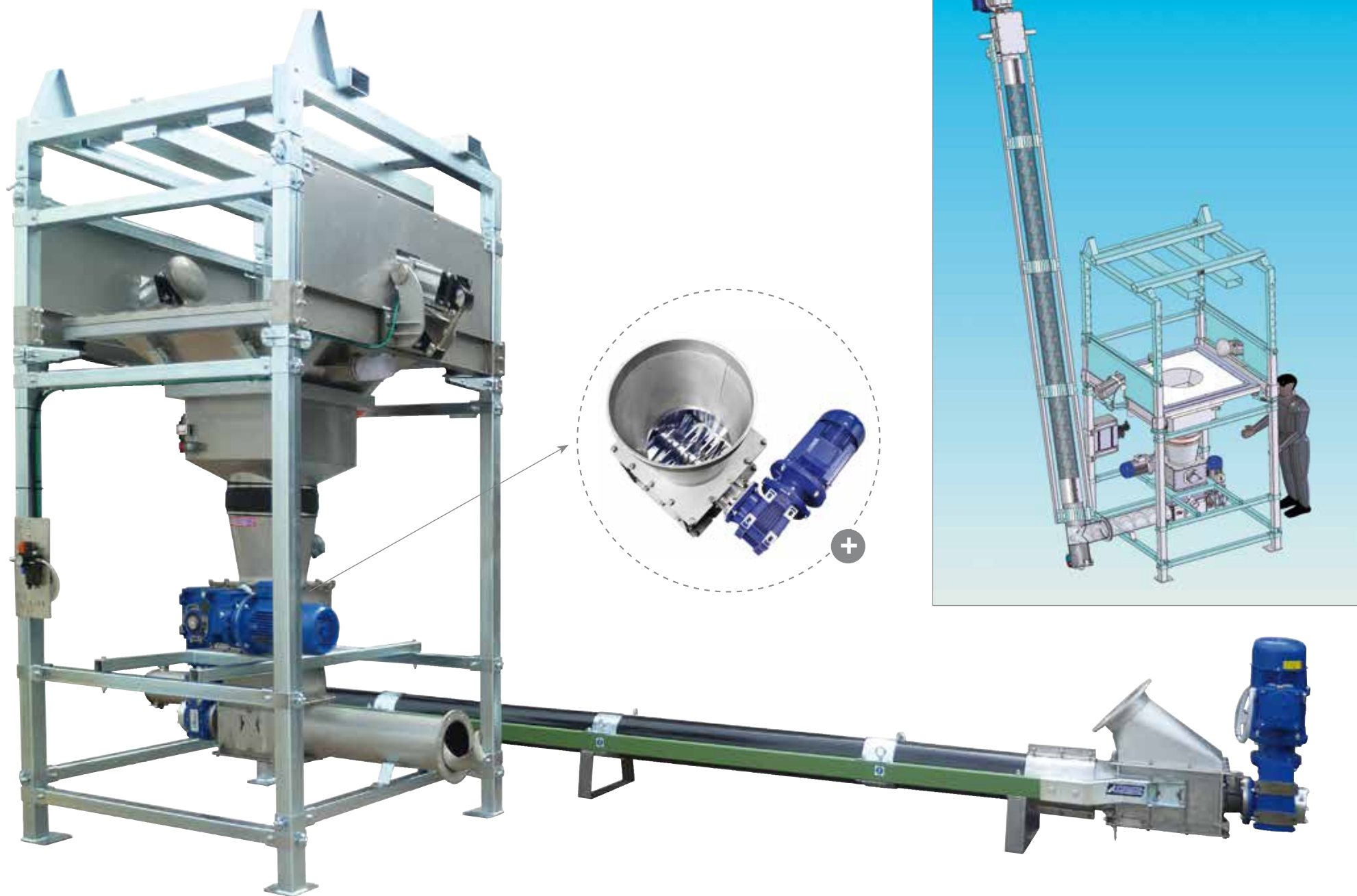
Bulk-Bag unloading system complete with lump breaker, shaftless screw conveyor (horizontal extractor and vertical elevator) type MAR 220 in ATEX zone 21 version
