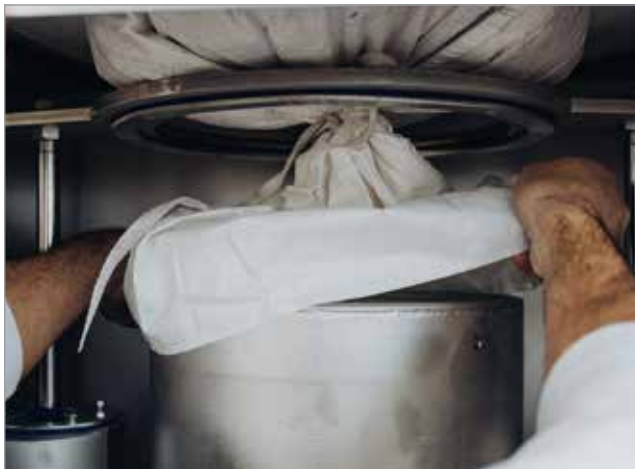
Pneumatic tightening system for dust proof bulk bag discharging
