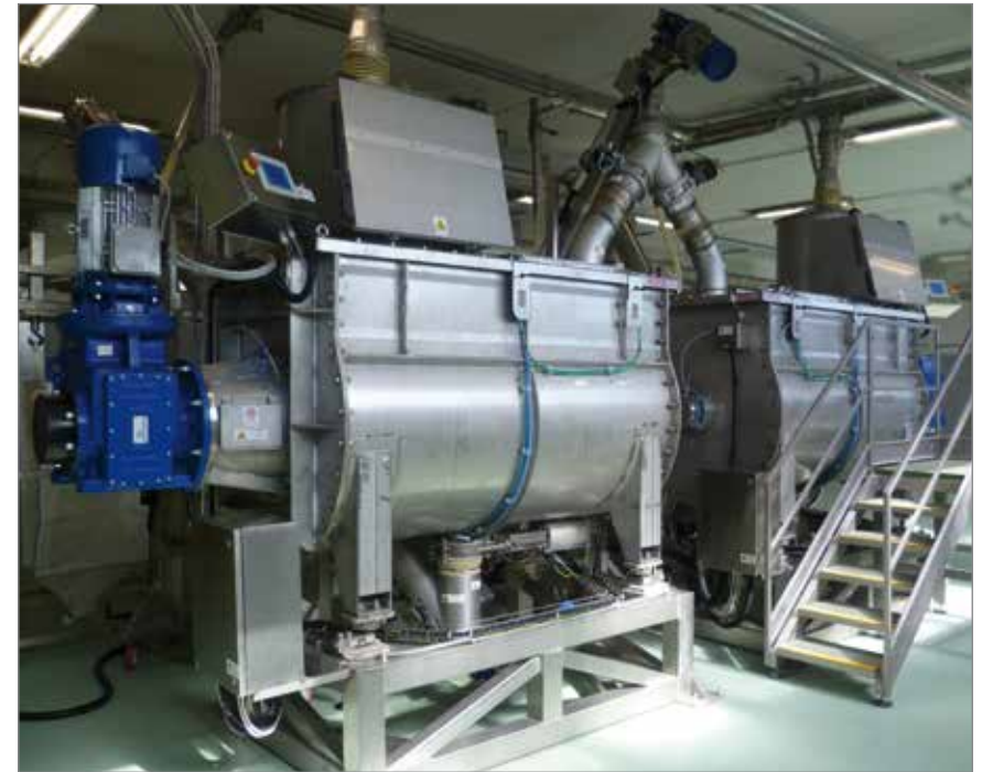
Plant complete with bulk-bag emptying unit, mixing unit and bag-filling unit supplied with weighing system
