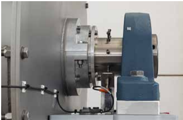
Ball Bearing end support with temperature and speed monitor
