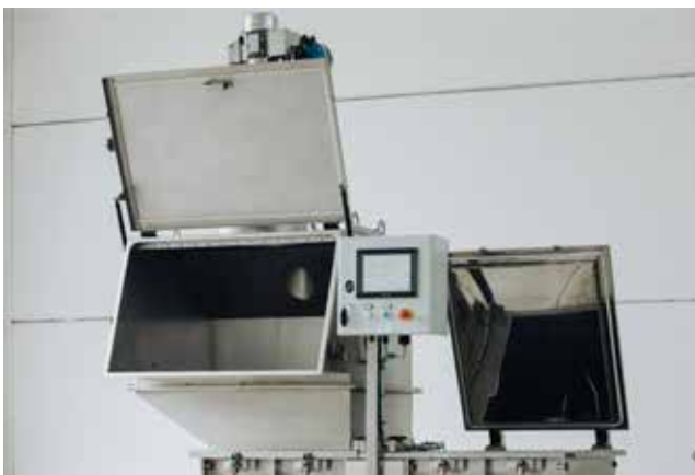
Sack tipping with dust extraction
