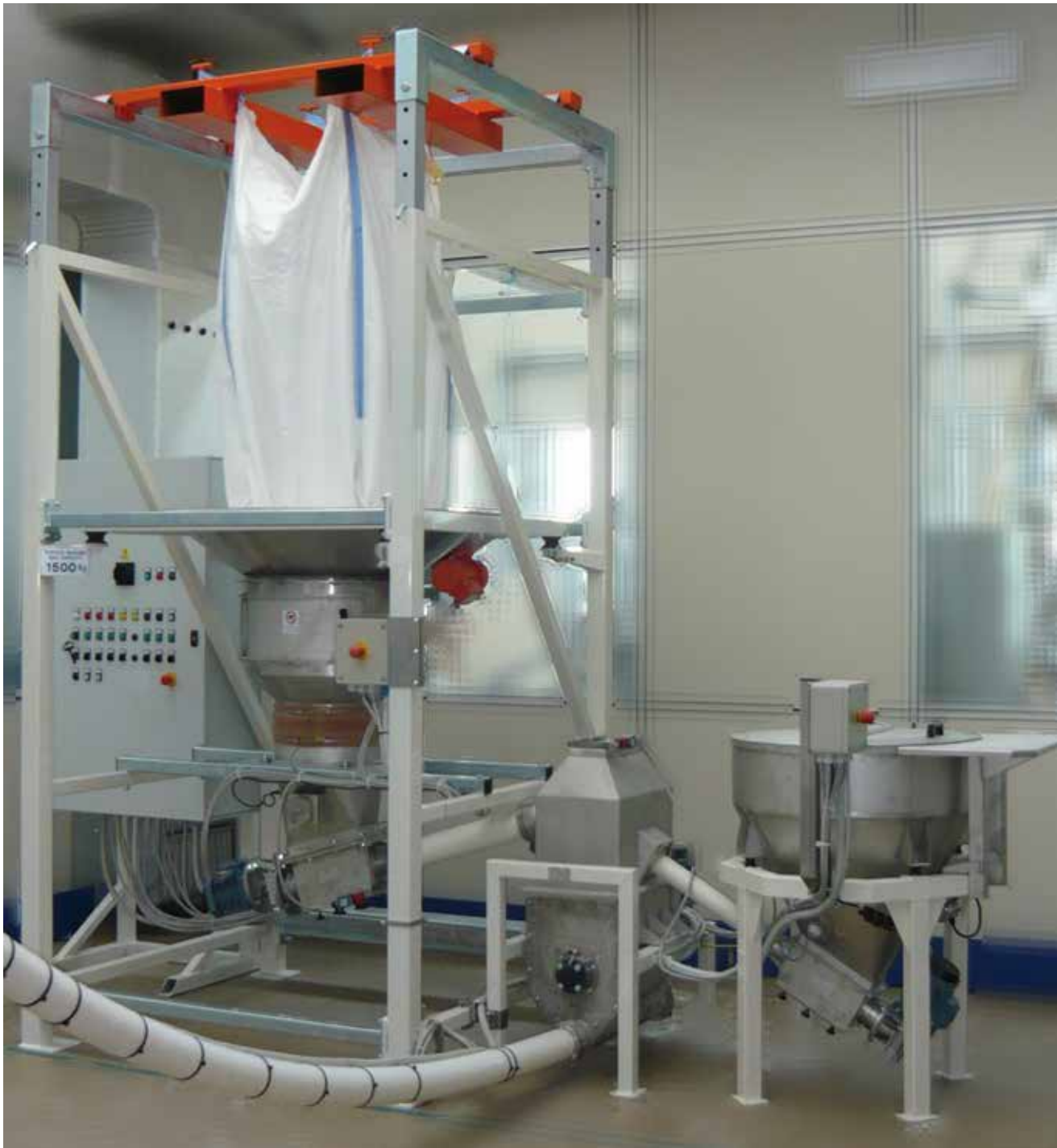
▲ Bulk Bag filling station with flexible screw conveyor
