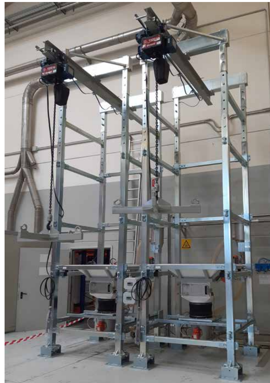
Bulk Bag emptying station on load cells and hoist lifting
