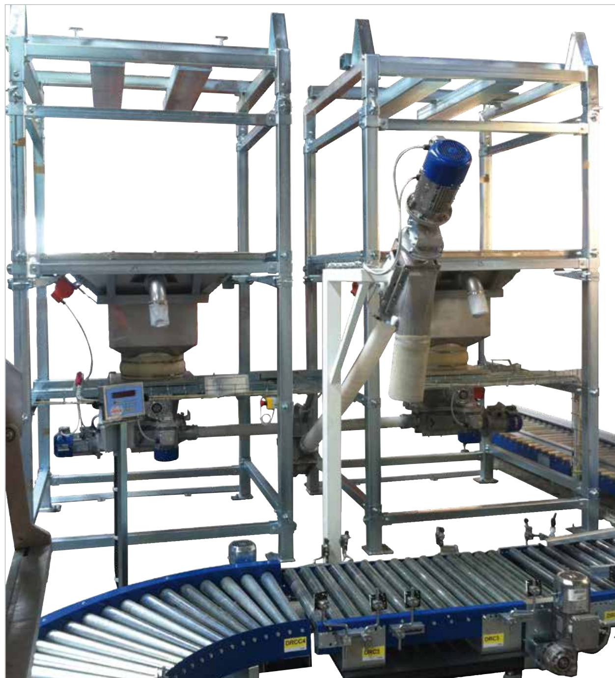
Bulk Bags discharging, continuous mixing of two different components and drums filling
