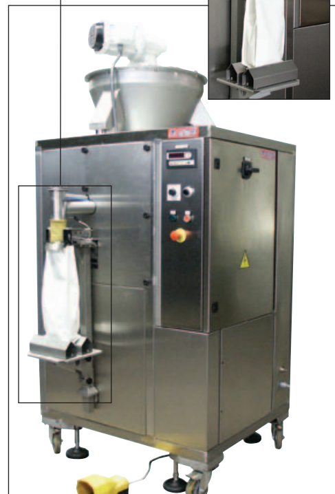
Screw filling with weighing device for small bags - drums from 0.5 to 10 kg
