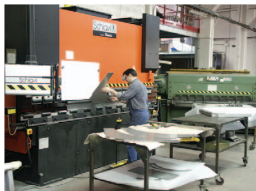
Numerically controlled steel sheets bending
