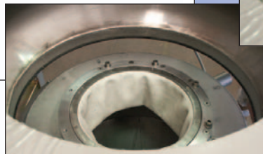
Iris valve for partial bulk bag unloading and slow bulk bag discharge
