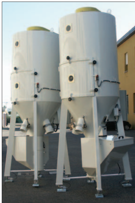
2000 lt Vertical Screw Mixers on load cells
