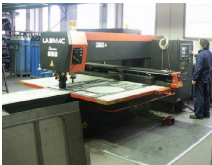
Processing sheets using laser cutting
