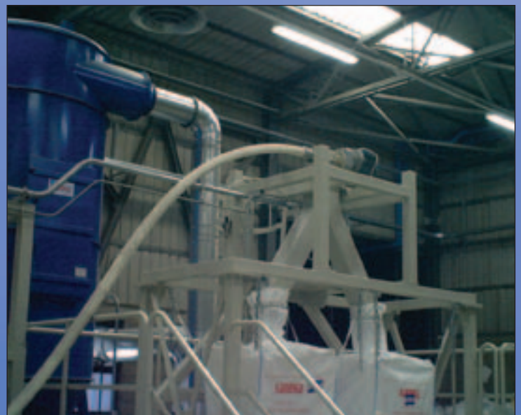
Bulk Bag filling station with flexible spiral conveyor
