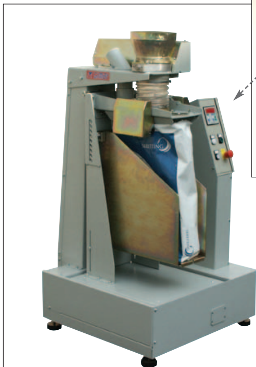
Scales with bag filling systems for granules into 25 kg open mouth bag
